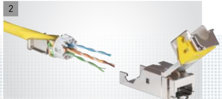
Pass the cable through the back of the wire housing
